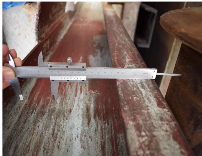
10#钟罩导轮与导轨间隙 45mm
